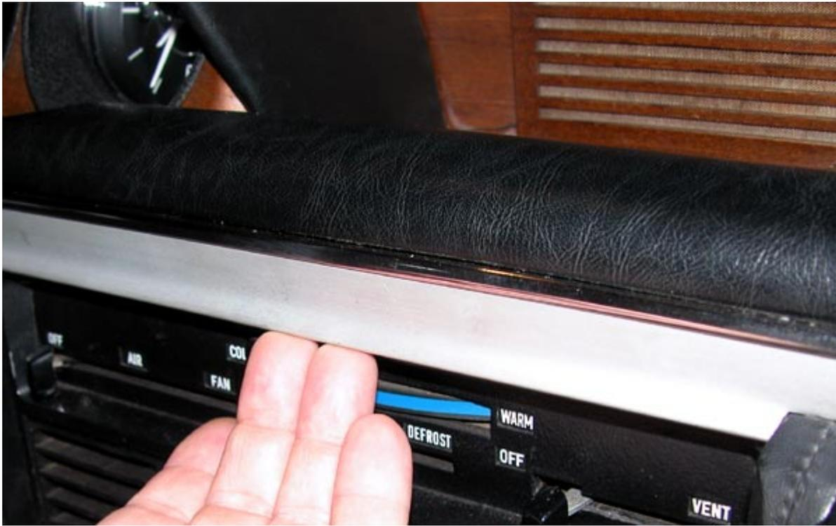
Once the trim is off you can see the big screws at each end, and the little screws that hold the lip onto the dash. With this part off it was much easier to get the sides of the console off.
