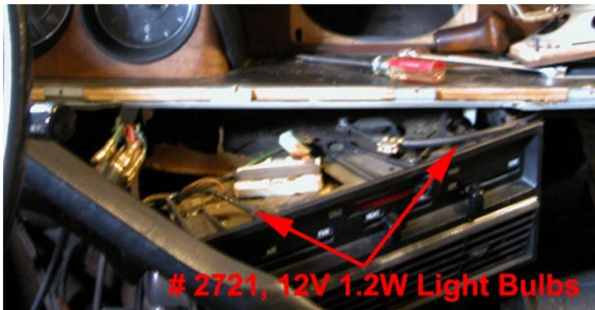
Once the console and lower dash panels are out of the way you can get to the nut and screw that hold the left side of the hood over the gauges, and to the two nuts that hold in the gauge cluster. You also need to disconnect the speedometer cable. My speedometer cable had a crew on collar that took a few turns to get off. I have been told that some only need a 1/4 turn to be free.
