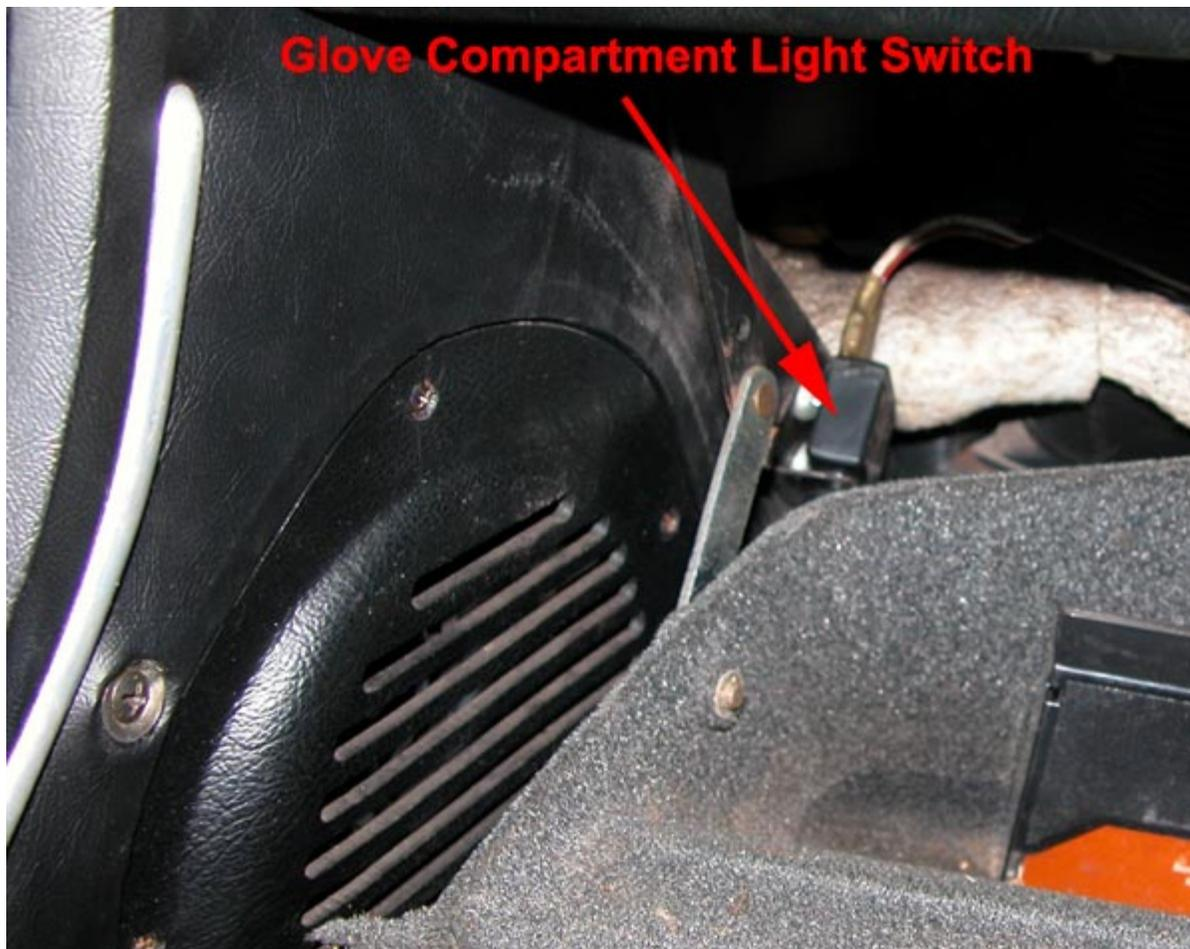
Console removal starts with removing the A/C air inlet covers (if you have A/C). Six little screws hold the cover on. The procedure is the same for both sides.
