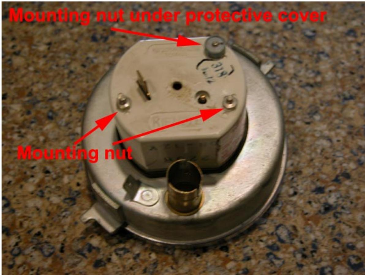
Once you get the plastic cover off it looks like the picture below. There is a metal strip that runs under the circuit board and is supposed to connect the 12V feed tab to the winding coil. The metal strip is connected to the tab on the coil by a small piece of very low temperature solder. Mine was melted and the metal strip had sprung away from the tab. I held the strip in place and used a little dab of solder to hold them together. The clock works great now.
