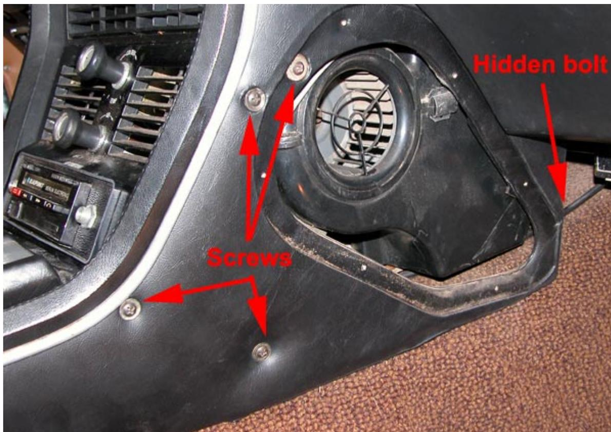
I removed the lip at the back of the dash shelf for more access. If you put your fingers under the trim and carefully pull, it will come off the dash. It is only held on by little push in studs. The stainless steel at the top of this trim comes off easily. Now is the time to polish it.
