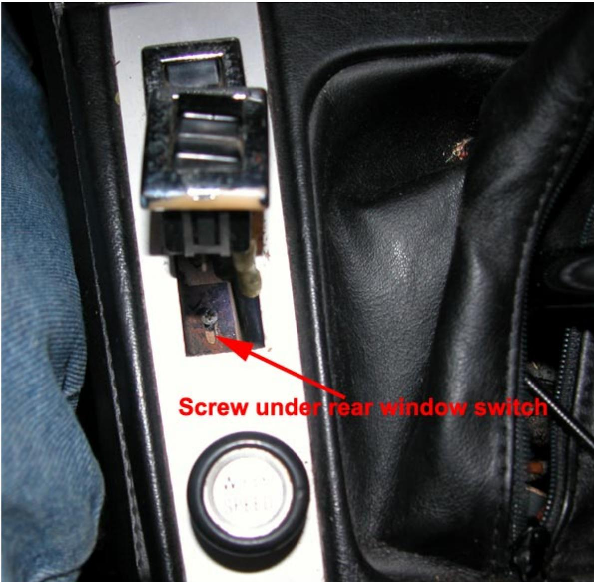
Shift into 2nd or 4th and you can lift the part of the console that incorporates the shift boot and switches over the shifter. You don't need to remove it, just lift it up for access.
