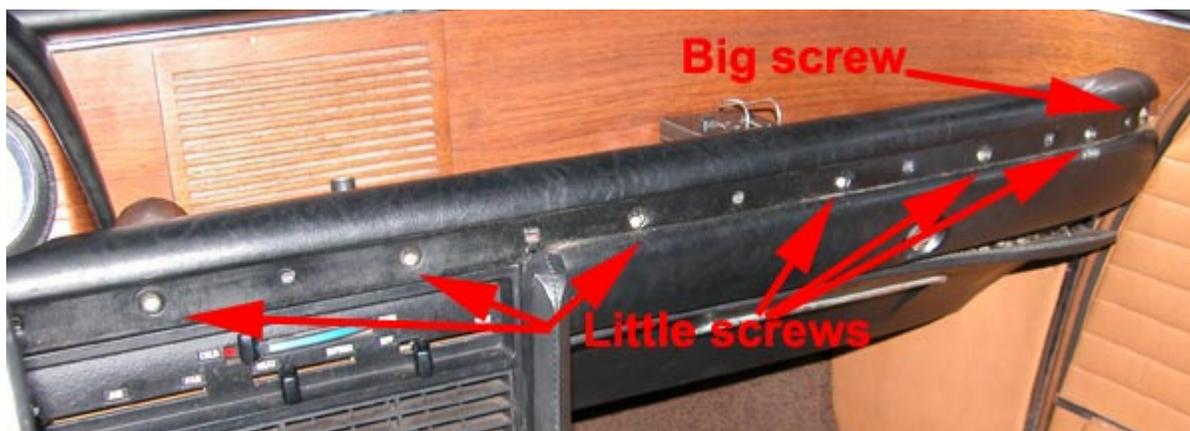
There is a screw under each rear window switch. Carefully lift out the switch. I found it easier to unzip the shifter boot and push the switches up from below. With the switch out of the way you can see the screws.
