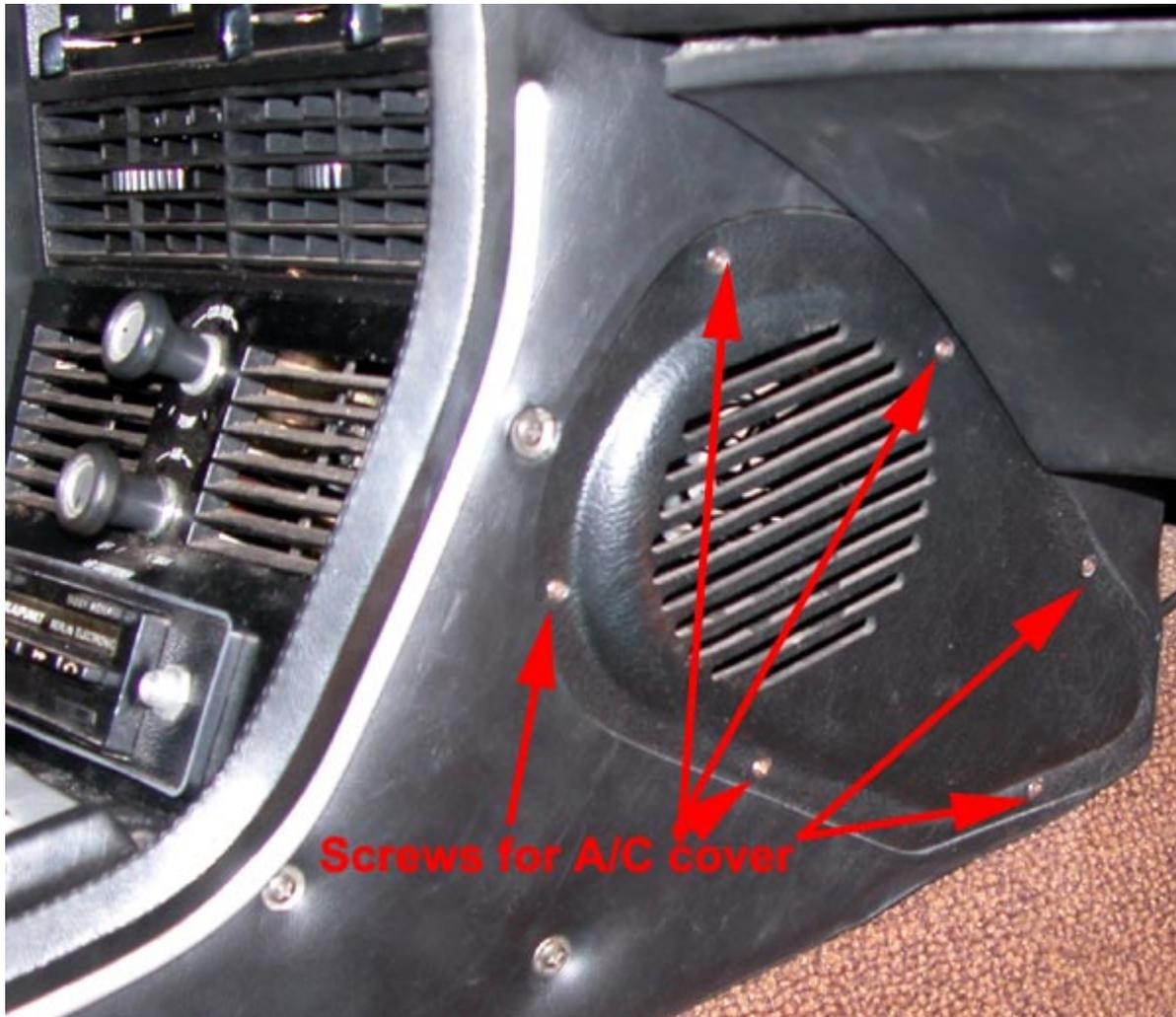
Then you need to remove four screws and one well hidden bolt. There is a nut on the bolt that is not attached to anything. Be careful or you will drop it and have a difficult time finding it.
